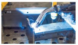
Fume extraction occurs at the weld gun and happens in sync with the rotation of the welding arm or boom. Wherever the gun goes, the fume extraction system goes within a 56' diameter circle. Efficient fume extraction is accomplished, with no time wasted on positioning equipment, which many times ends up being in the way and cluttering up the workspace.
