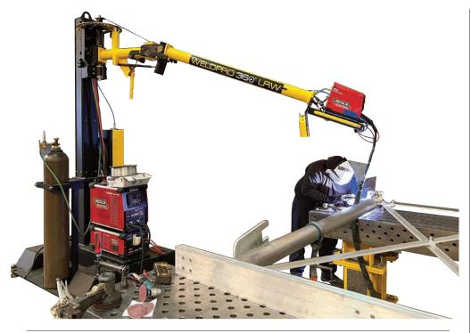
WELDPRO 360 LRW-10ML Mig Welding Arms reduce or eliminate non-arc time welding-related tasks, shop floor clutter, and employee safety issues. This arm provides complete coverage anywhere with-in a 40' diameter semi-circular welding zone. The welding arm's main pivot assembly mounts to your existing building column, freestanding column or the optional mobile base and column assembly.
