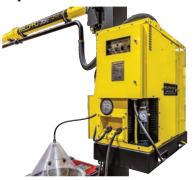
WELDPRO 360 LRW Hi Vacuum Fume Extraction systems are integrated with the welding arm. Available in boom mount or mobile.
