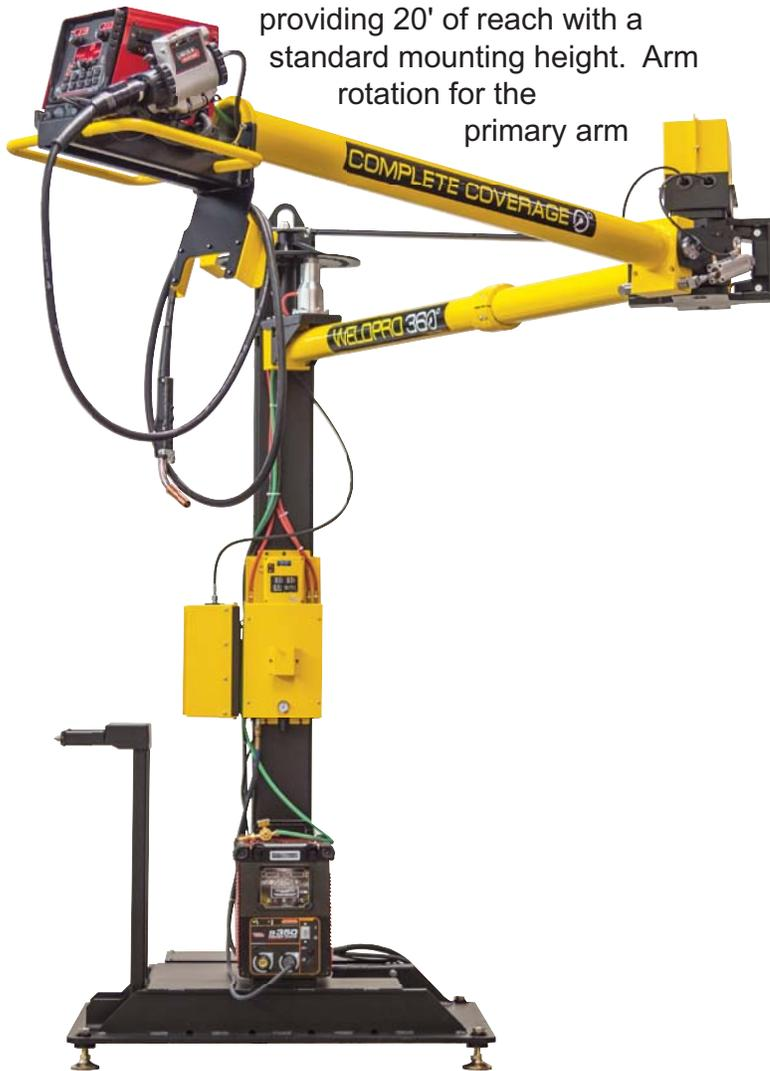
and raise/lower functions of the secondary arm are controlled with a wireless remote that hangs on the operators belt. The arm control requires only 90 PSI of compressed air and a 120V electricity to operate.
