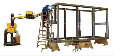
WELDPRO 360 LRW-18 Mig Welding Arms reduce or eliminate non-arc time welding-related tasks, shop floor clutter, and employee safety issues. This arm provides complete coverage anywhere with-in a 56' diameter semi-circular welding zone. The welding arm's main pivot assembly mounts to your existing building column, freestanding column or the optional mobile base and column assembly.
