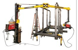
This eliminates wasted time walking back and forth to the welder to change weld settings. Welding wire conduit liner, power cable, gas and air hoses are all contained within the tubular arms eliminating safety hazards and shop floor clutter. This makes for a neat, clean, organized shop.
