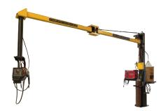
The WELDPRO 360LRW-18P Mig Welding Arms reduce or eliminate non-arc time welding-related tasks, shop floor clutter, and employee safety issues. The welding arm's main pivot assembly mounts to your existing building column, freestanding column or the optional mobile base and column assembly. They provide complete coverage anywhere with-in a 56' diameter semi-circular welding zone.
