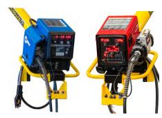
This eliminates wasted time walking back and forth to the welder to change weld settings. Welding wire conduit liner, power cable and gas hoses are all contained within the tubular arms eliminating safety hazards and shop floor clutter. This makes for a clean, organized shop.
